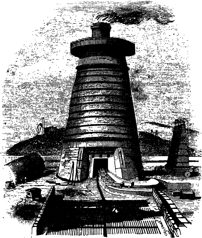
Fig. 203. The Tapping of the Blast Furnace.
